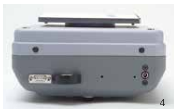
1. Balance model Cent 2. 3. Keyboard, Square Pan 4. Rear side with RS232 5. Balance model Cent 203
